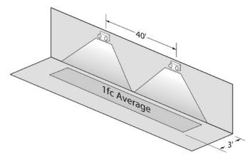
Using multiple units with optional 25 watt MR16 lamps mounted at a typical 7.5' delivers 50' center-to-center spacing on a 3' wide egress path.
