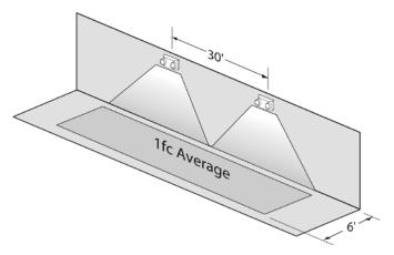
Using multiple units with optional 25 watt MR16 lamps mounted at a typical 7.5' delivers 40' center-to-center spacing on a 6' wide egress path.
