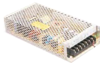
StarStrand 150w Direct Wire Driver 53277 7.75"L x 3.75"W x 1.5"H • 120V/240V input • 12V, 12.5 Amp output • Includes one 72' output cord
