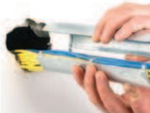
Ready™ Sleeve convenience for existing cable installations. Split sleeve and two-piece wall plates allow sleeve to be assembled around cables and locked into the wall or floor. Available in 1" (33 mm OD), 2" (60 mm OD), and 4" (114 mm OD) sizes.
