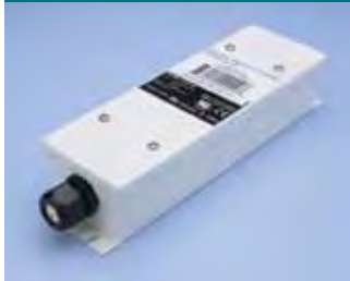
LEDDR-12-60W 10.25" x 3" x 2" Class 2 1 circuit at 60 watts for 12VDC RU Component indoor/outdoor listed
