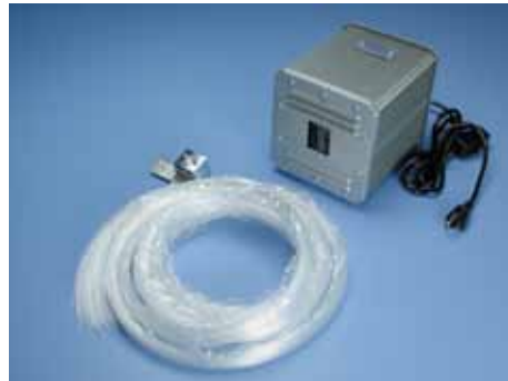
GP-35B-12' 35W Illuminator with a harness of 160 Fibers in a 12' length. 7" x 5.5" x 5.75" - 35 watt Halogen bulb.
