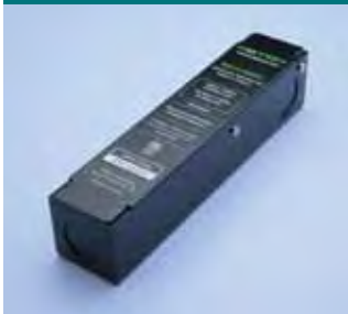
TECLT-12-60 6.5" x 1.5" x 1.5" Class 2, 1 circuit at 60 watts for 11.7VAC
