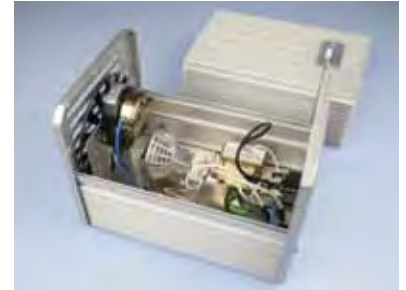
GP-5-12' Interior showing 5 watt LED MR-16 bulb
