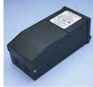
TR-12-300 or TR-24-300 10" x 4.25" x 3.6" 2 circuits at 150 watts each for 12VAC 1 circuit at 300 watts for 24VAC
