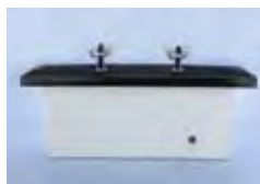
Concrete Cap installed in fixture
