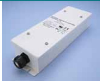
LEDDR-24-120W 11.6" x 3.6" x 2.25" Either 1 circuit at 90 watts, or 2 circuits at 60 watts for 24VDC RU Component indoor/outdoor listed
