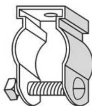
6H-B Series with bolt and hex nut Fig. 2
