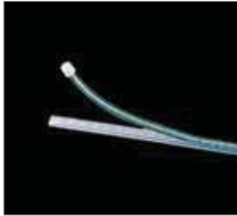
When straight line installation is needed, the channel (NFL-509) is required. Drill holes in channel and nail or screw channel onto surface.
