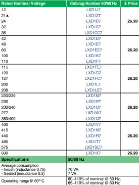
Voltage for special coils fitted in contactors with serial timer modules, with 24 V supply.
