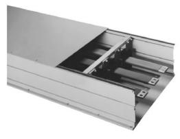
Transformer/Generator Connection – This type of termination should be priced whenever the bus is connecting to a transformer, generator, motor, switch or any connection where the bus bars are connecting to porcelain mounted equipment terminals. It will include the same components as a flanged end plus one set of flexible braid type connectors and a terminal box (if required).
