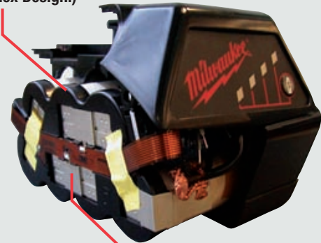
4-Point Battery Strap Welds Per Cell Ensures Job Site Durability
