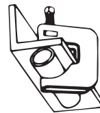
C-247 Beam clamp supports pipe.
