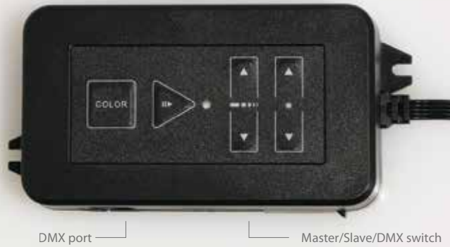
Wired controller (required) LED-TC-CTR-MSD
