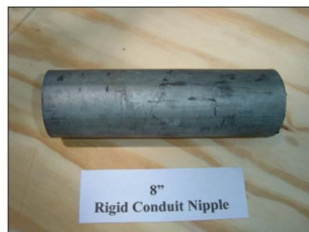
2. Remove 1" piece lengthwise from the nipple.
