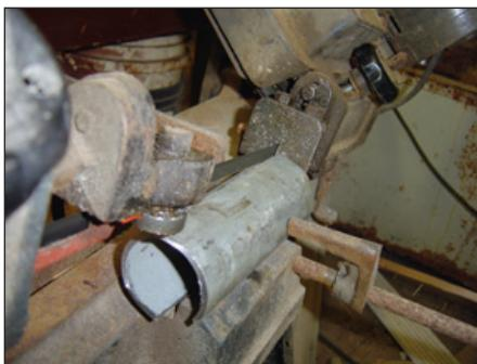
3. Cut the remaining nipple lengthwise in half.
