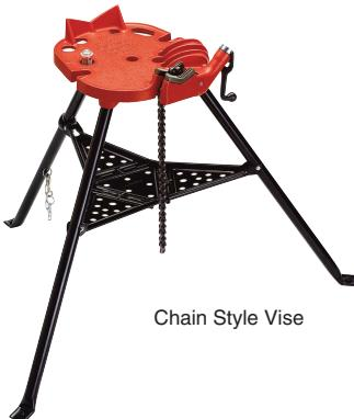
If a chain style vise is to be used, the chain as well as the jaw inserts will tear the PVC coating when the threading force takes place.
