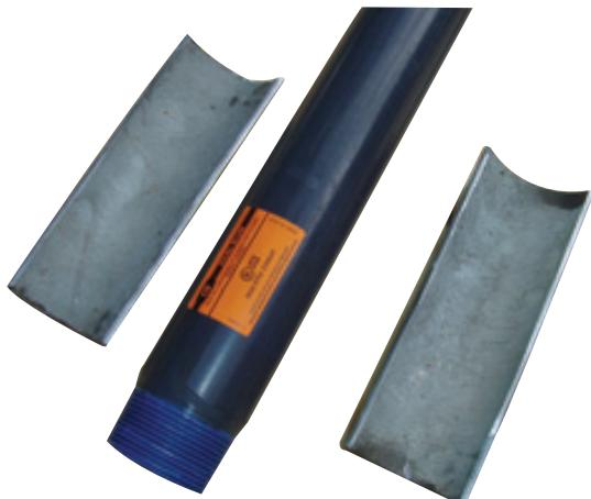
The vise jaws and chain will now clamp around the shells and hold the conduit without damage.
