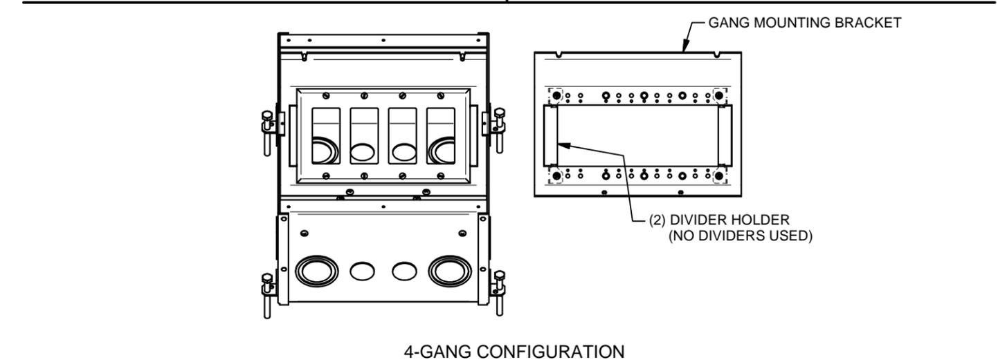
**BOTH GANG MOUNTING BRACKETS ARE IDENTICAL, AS IS THEIR CONFIGURATION CAPABILITY**
