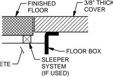
NOTE: FOR 3/8" THICK COVER LOWER TEMPORARY COVER AN ADDITIONAL 1/4" FROM FINISHED FLOOR DIMENSION OR USE SHIM KIT
