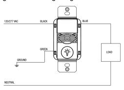
Three-way wiring diagram: Lights will turn OFF automatically when sensor that detected motion last, times out.
