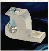
Lay-in connectors offer the ultimate in flexibility. Excellent for grounding and continuous loop applications. Made of 6061T-6 aluminum alloy. Tin plated for low contact resistance. Suitable for use with both copper and aluminum conductors. Rated 600 volts.
