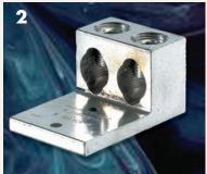
Set screw connectors that will accept either one or two wires. Made of 6061T-6 aluminum alloy. Tin plated for low contact resistance. Suitable for use with both copper and aluminum conductors. Rated 600 volts.
