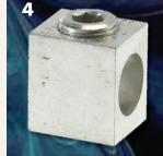
Made of 6061T-6 aluminum alloy. Tin plated for low contact resistance. Suitable for use with both copper and aluminum conductors. Rated 600 volts.
