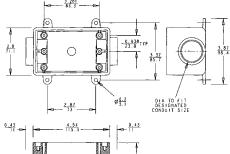
For through terminations where large devices or additional wiring capacity is required.
