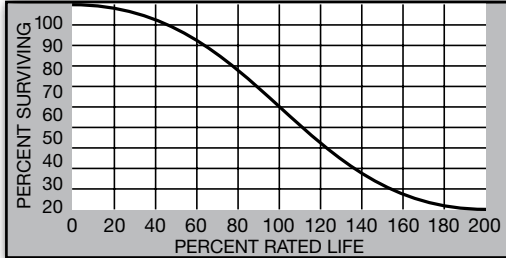
TYPICAL FLUORESCENT LAMP MORTALITY
