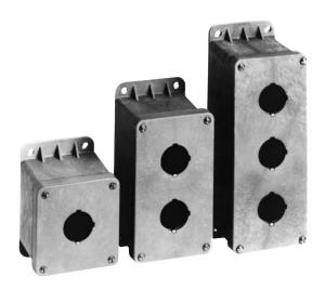
Wall mount pushbutton enclosures are molded from grey engineered thermoplastic material that is resistant to most corrosive agents. Universal pushbutton holes are designed to accommodate all standard oil-tight pushbuttons, switches and pilot lights. A grounding plate is included on the cover. Auxiliary devices must be rated for appropriate NEMA applications...
