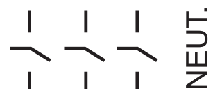
Four-wire SN, 240 Volts AC, No Fuse
