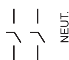
Three-wire SN, 120/240 Volts AC, No Fuse
