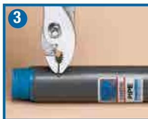
In **Step 3**, the tab is pulled perpendicular to the conduit with a pair of pliers. The plastic tab will tear off rather than having any peeling effect or the coating separating from the substrate.
