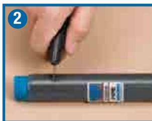
**Step 2** calls for the edge of the PVC that was cut on the perpendicular to be carefully lifted to form a plastic tab.
