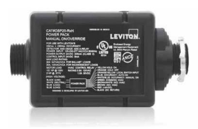
Containing both a 24VDC supply and a 20A line voltage relay for most models, the Leviton compact Power Pack provides low voltage power and line voltage control for Leviton Occupancy Sensors. Versions include Auto-ON and Manual-ON inputs for occupancy sensors, Hold-ON and Hold-OFF capabilities, and a local input for momentary or maintained dry contact switches.
