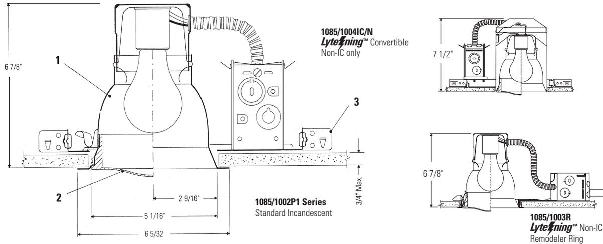
Complete Fixture consists of Reflector Trim & Frame-In Kit. Select each separately.
