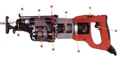
**Easily Accessible Dial Speed Selector** Switch matches the correct speed with application for improved control.
