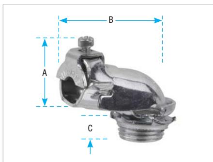
The angle clip gives secure mechanical grip that tightens under tension or vibration. Throat is long enough to install in cast housing knockouts. The 3/8 in. and 1/2 in. sizes are of steel construction. The 3/4 in. and larger sizes are malleable iron.
