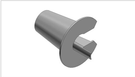
Anti-short bushings are made of smooth plastic, and designed to protect conductor insulation from rough edges of armoured cable and flexible metal conduit
