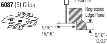
Slotted Grid Ceilings such as Donn Fineline and Chicago Metallic Ultraline 3500 and 3600. Use two per 2' and 4' track, three per 8', and four per 12' track.
