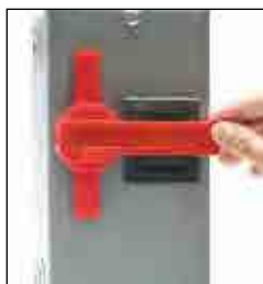
Slide Stop Bar into position over breaker
