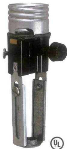
ADJUSTABLE TURN KNOB 22118 - REMOVABLE KNOB STANDARD BASE 1/8-IP HICKEY 250 WATTS 250 VOLTS HEIGHT ADJUSTABLE FROM 4" - 5 1/4"
