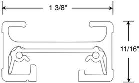
One-circuit Trac-Master™ sections are available as surface mounted track or may be suspended from ceilings with pendant accessories listed on page 3.
