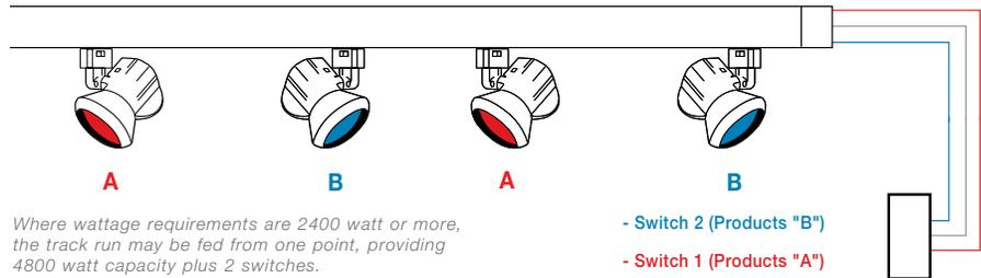
*Where wattage requirements are 2400 watt or more, the track run may be fed from one point, providing 4800 watt capacity plus 2 switches.*
