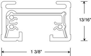
Juno two-circuit Trac-Master™ features a sleek low profile design with the flexibility of individual circuit control for combining dual lighting effects along a single track.
