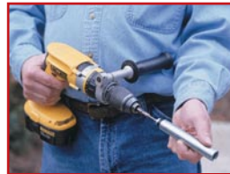
2. Snap on drive sleeve and drive in anchor
