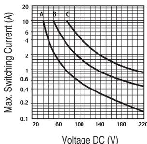
**Breaking capacity for DC1 load at 1,800 cycles/h.**
