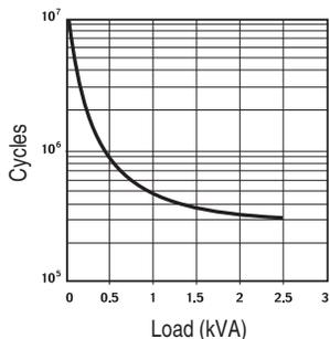
**Contact life vs. AC1 load at 1,800 cycles/h**
