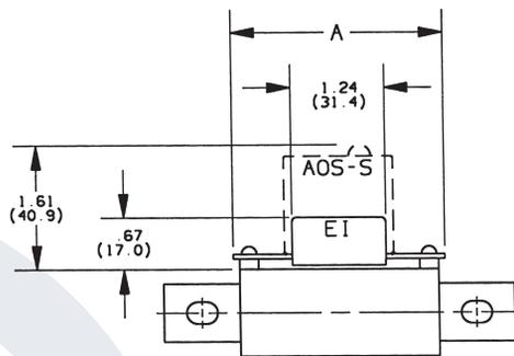
Note: Fuses with the EI option are designed to work with the AOS-S or AOS-Q add-on switch, which is ordered separately. See page J6 for details.
