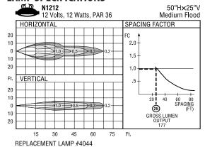
Spacing Factor: Indicates the proper spacing between lamps to the chosen illuminance level (fc)  $\pm$  20%. Footcandle Curves: Show distances in feet and isocurves in footcandles.
