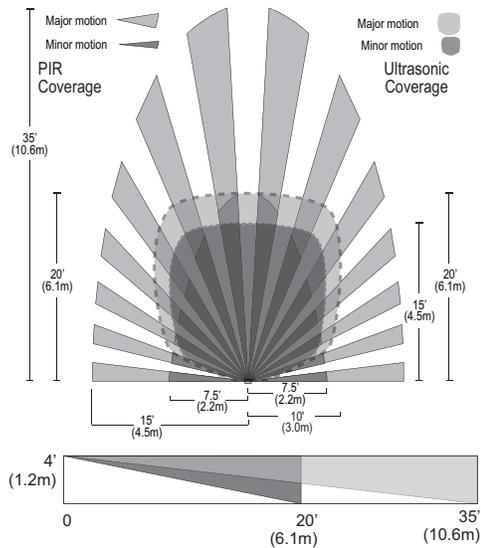
For best performance, Wattstopper recommends using this sensor in spaces no larger than 18' x 15'.
