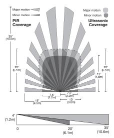
For best performance, Wattstopper recommends using this sensor in spaces no larger than 18' x 15'.
