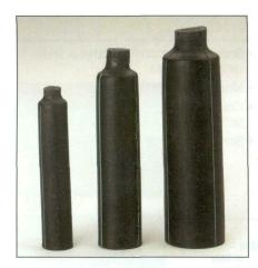
Seals and insulates cable ends at a 600V rating. Installs fast, while providing insulation resistance to moisture corrosion and abrasion. The extra thickness at the tip of the end cap prevents sharp ends of the cable from puncturing the seal.
