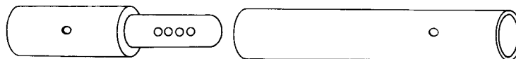
400 Amp 0.84" Solder Well Wire Terminals. Solid Copper Contacts with Four Spring-Loaded Borosilicate Bearings.
