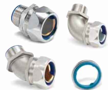
T&B 304 Stainless Steel Liquidtight Fittings — Straight (top left), 45° Angled (bottom left) and 90° Angled (top right). 5262 Series Sealing Ring Gasket (bottom right) sold separately.
