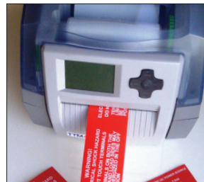
Using the suggested white ribbon, white text can be printed on red or black vinyl or a black ribbon can be used to print on the white vinyl.
