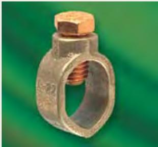
This heavy duty ground rod clamp replaces all existing ground rod clamps, eliminating the need to stock several different sizes and types. UL listed for direct burial in earth and concrete, the heavy duty construction enables it to handle large ground wires up to 1/0 AWG – much larger than a standard ground rod clamp. Suitable for: 3/8", 1/2", 5/8", 3/4" ground rods.
