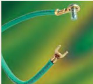
Green insulated conductors supplied with a spade terminal on one end and a ring terminal with a captive green-dyed screw on the other end. 65 strand #12 awg and 41 strand #14 awg for maximum flexibility. Available with round, hex head or combo screw.
