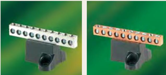
Made from either high-strength aluminum alloy 6061-T6 or high-conductivity copper as indicated below. The base is made from high-strength glass-filled polyester. Aluminum connectors are dual-rated for use with aluminum or copper cables.
