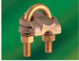
Made of high-copper-content alloy for grounding to 1/2" - 1" ground rods and ground pipes from 1/4" - 3 1/2" in parallel or 90° position. Suitable for direct burial in earth and concrete. Nuts and lockwashers are silicon bronze.
