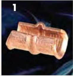
These taps ensure positive, all-around compression with low resistance and high pull-out values. Made of high conductivity copper, they satisfy the requirements of NEC250-81 and 250-91 for connecting to the grounding electrode system. Rated for 600 V applications.
