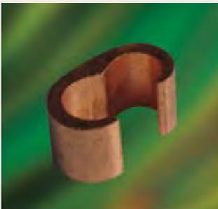
Copper "C"-Taps are range-taking compression connectors made from high conductivity copper alloy. They are used for making tap or parallel copper connections from 8 SOL to 4/0 STR conductors. C-Tap connectors provide consistent reliability with heavy wall construction that prevents relaxation of the joint after installation. Installation time is reduced because of its "C" shape. UL CU486A, 467 suitable for direct burial and CSA rated Electrical and Grounding.
