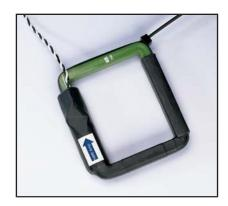
Using a flathead screwdriver, press the tab on the nylon clamp to open the current sensor assembly.
