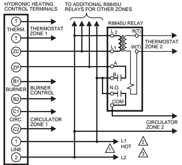
Fig. 3. R8845U schematic diagram for multizone, hydronic heating system (applies for any number of additional zones).
