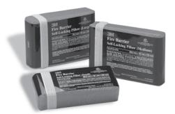
Self-contained, highly intumescent pillows are designed to firestop a wide variety of through-penetrations including cable trays, conduit and blank openings. Interlocking strips hold pillows securely together yet release easily for retrofit or reuse—just remove and replace pillows as needed.
