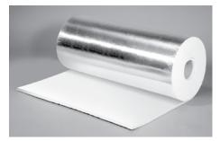
This endothermic wrap is designed to block heat penetration by chemically absorbing heat energy. When exposed to high temperatures, it keeps heat out by releasing chemically bound water to cool the outer surface.
