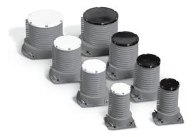
These firestop devices are designed to make firestopping through concrete easy and affordable. With models available to accommodate plastic or metallic pipe, 3M<sup>™</sup> Fire Barrier Cast-In Devices are installed prior to the concrete pour (attaching directly to the wood forms) and can be adjusted to various concrete depths.
