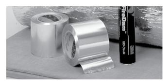
3M Interam Tape T-49 is an adhesive-backed aluminum foil tape designed to seal the cut edges of 3M Fire Barrier duct wrap and interam mats to complete the total encapsulation.
