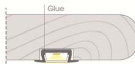
G Recessed Mounting into a Mitered Groove using a flanged Channel
