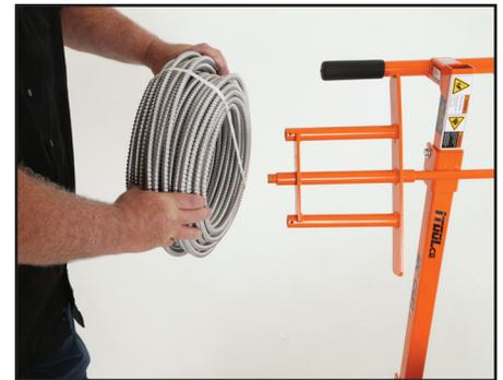
Cable Mate holds one 250' coil of MC.
