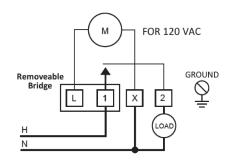
For separate motor terminals remove bridge from terminal L & 1.
