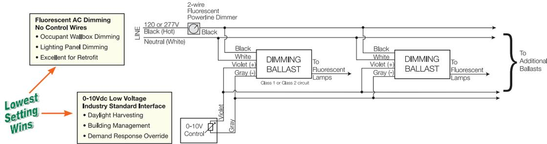
**Wallbox Style 2-wire Powerline Control Wiring Example**
