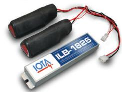
IOTA's constant current emergency LED drivers provide higher wattage output and external battery mounting with optional cold-weather performance. Two units offer output voltages of 18-26VDC up to 20W (ILB-1826) or 27-30VDC up to 24W (ILB-3020). Battery profile options vary depending on model. Refer to complete specifications for detailed profile data.
