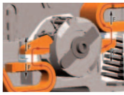
Figure 14: Rotational contact mechanisms use the repulsive magnetic field forces in such a way as to greatly accelerate the switch's opening time in order to achieve a higher degree of current limitation.
