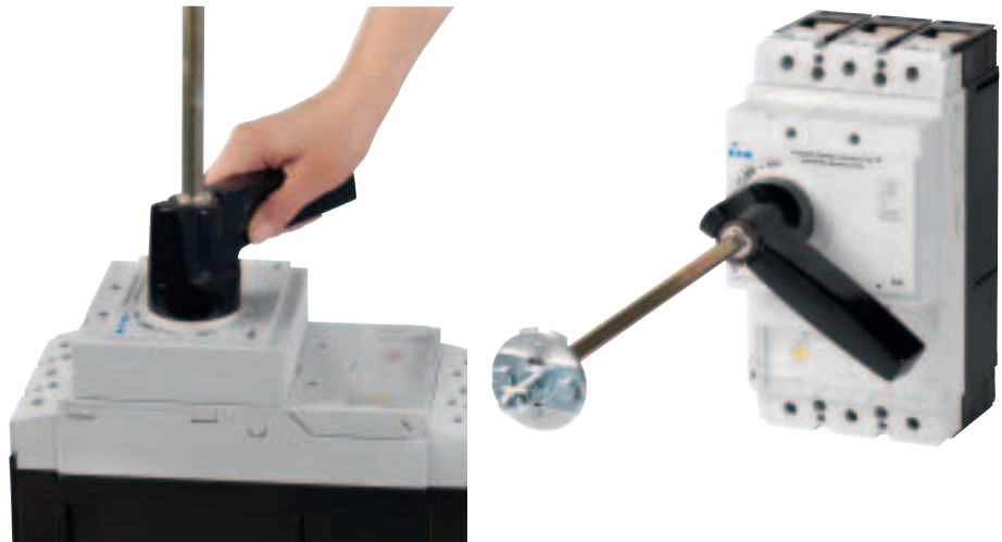
Figure 34: The photo on the left shows a supplementary handle (in the ON position) for a Frame Size 2 switch. The right portion of the photo shows the slightly larger handle required for Frame size 3 and 4 switches.
