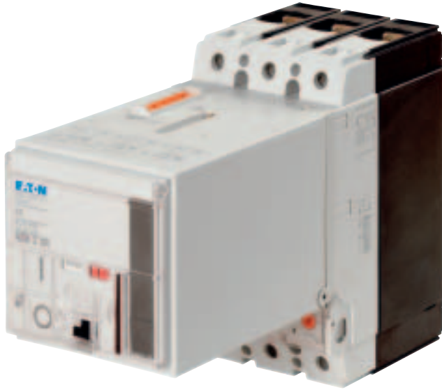
Figure 29: Electrically motorized drives allow ON-OFF operation of the switch from a remote location. The motor drives utilize a stored energy spring mechanism, which enables a quick closing of the switch at the application of an electrical signal. The opening and spring loading operations are carried out by the motor. The motor drives can also be mechanically actuated at the switch. In cases where the opening action of the switch via the motor would be considered too slow, usage of voltage trip accessories can be introduced to quickly trip open the switches.
