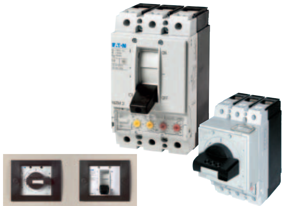
Figure 28: Versions of operating handles which remain in contact with the switch. The handles can be operated through a cut-out in the door, which is suitably framed using the molded cut-out frame accessory (Type NZM...XBR). The handles can be directly padlocked if desired. Currently, the padlockable accessory for the toggle operator is not certified for North American versions. These through-the-door operating handle versions are normally associated with additional electrical interlocking provisions. This type of mounting would not be generally considered acceptable for the supply circuit disconnecting means per the North American Industrial Machinery standard NFPA 79 simply because the environmental rating of the handle and molded frame assembly would not be sufficiently adequate for that application.
