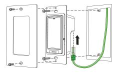
LMDM-100 Dimming Wall Switches fit in standard single gang boxes.
