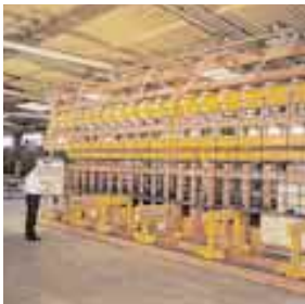
Cable tray testing machine
