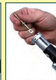
Insert 1/4" x 3" acoustical lag screw into top slot.
