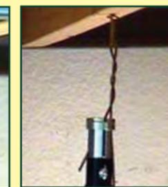
Rotate the tool again to twist the wire. Telescoping Pole Tool may be turned by hand or by using a 1/2" variable speed drill. Caution: if using drill, do not grip pole tightly with hand, but allow it to turn loosely.
