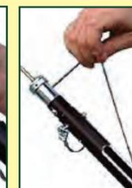
Insert wire into side of slot, through the hold in the lag screw. Then bend the wire end down.
